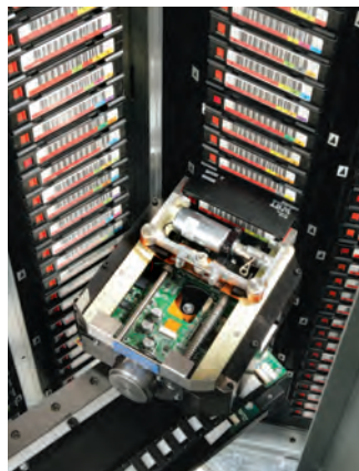
Robotics never leave the LRM to access cartridges in the MEM, insuring fast access times and high reliability.
