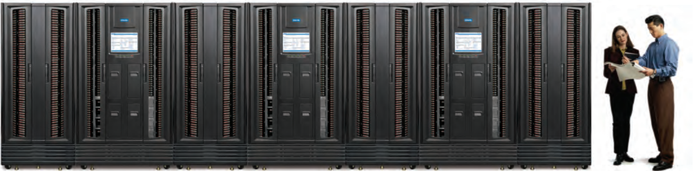
Configurations containing up to 4 LRMs and 5 MEMs store over 9,600 tapes.
